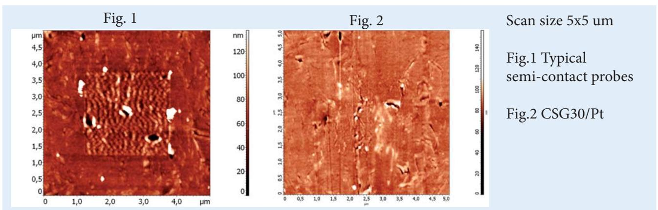
As the result of experiment there are some surface changes after using the typical semi-contact probes for conductivity measurements, but there are no destructions after CSG30/Pt tip using.
