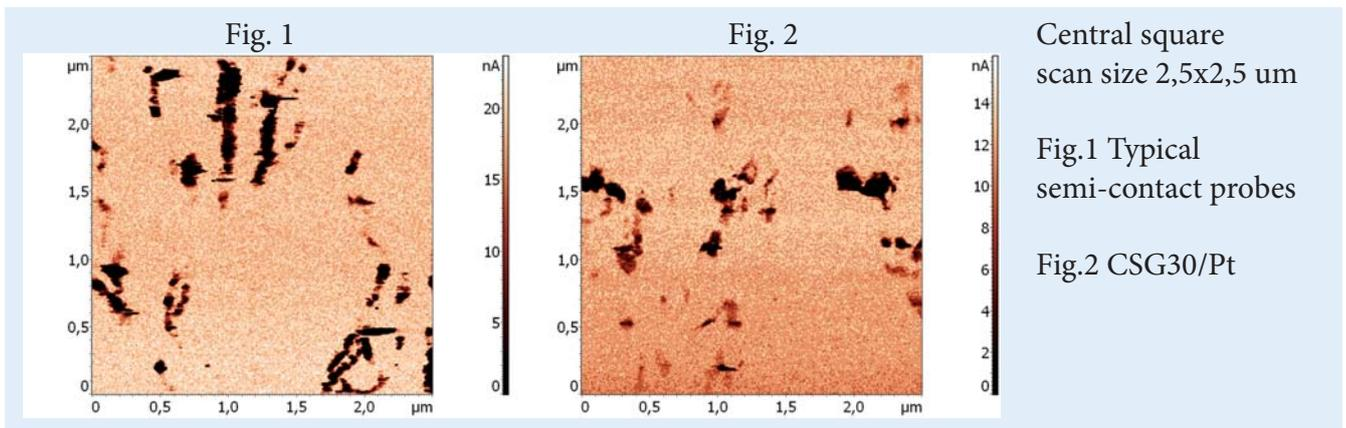
Step 3. Semi-contact mode - checking the surface changes after the contact mode
